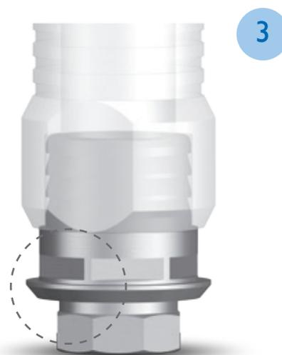
For casting use high-melting cobalt-chrome alloy. Devest gently with ultrasound, water jet, pickling acid or a glass-fiber brush. To remove the oxide layer use glass beads ( $50\ \mu\text{m}/2\sim 4\ \text{bar}$ ). Be aware of danger of damage of the inner configuration and of the prefabricated connection to implant. Protect carefully the connection to implant during all manipulations with the abutment.
