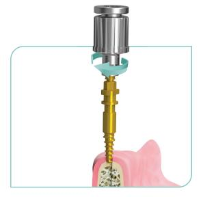
Start the insertion manually without using the ratchet.
